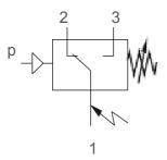
The pressure switch is connected via the 3-pin terminal in the terminal compartment (type of protection Ex e) and lying in the interior of the separate protective conductor terminal.
