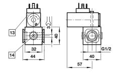
13 Pressure switch is not in scope of delivery 14 Alternative G1/4 ports plugged
